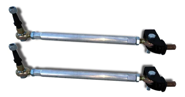
LG Motorsports HD rear tie rod kit is designed to offer a full range of travel as a bump steer kit and beef up the tie rod where the factory left off. Angle adjustments can be made at the inside and outside of the rod and use Left hand / Right hand ends for quick and easy toe adjustment changes. The inside mount is offset to allow more clearance for aftermarket coil overs and other suspension changes. Works with OEM and LG Billet spindles.
