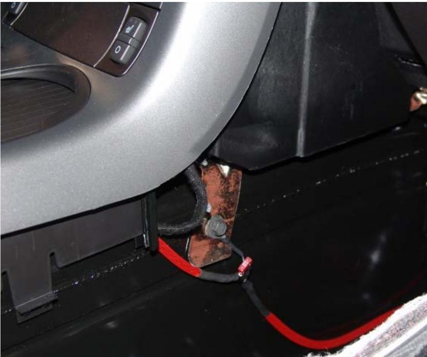
**Figure 4: Installing the ground strap**
