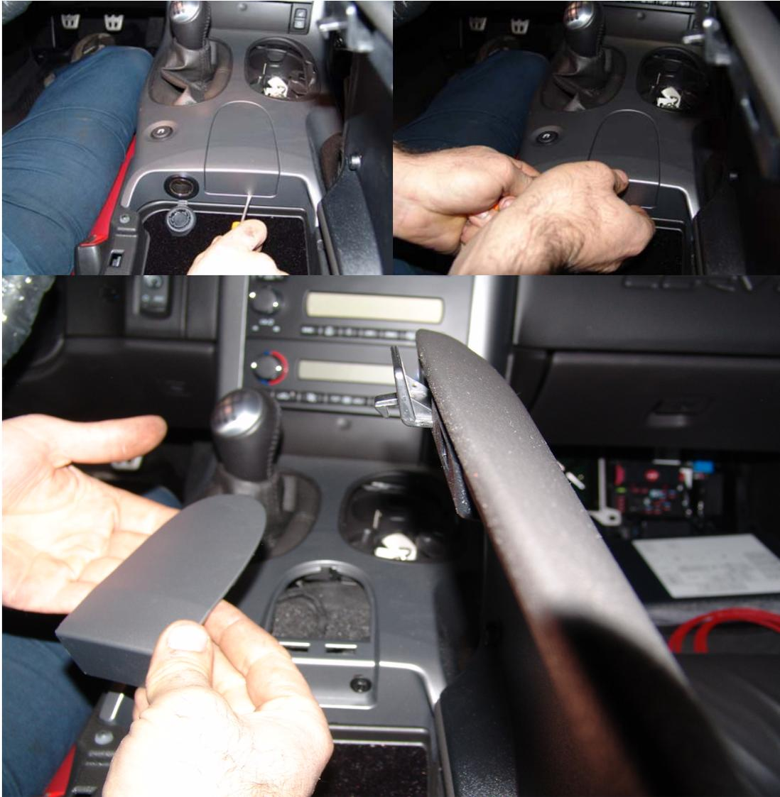
Figure 1: Removal of center console piece
