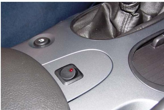
**Figure 7: round lighted switch installed**
