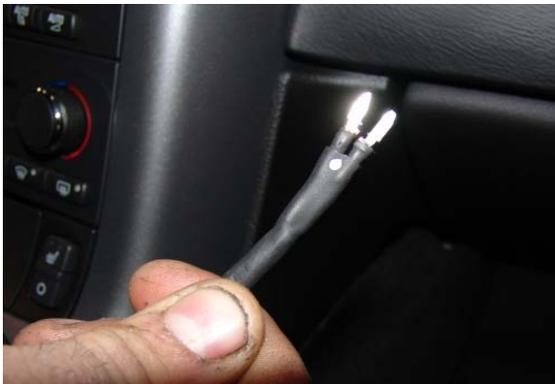
**Figure 6: Fuse tap with marking**
