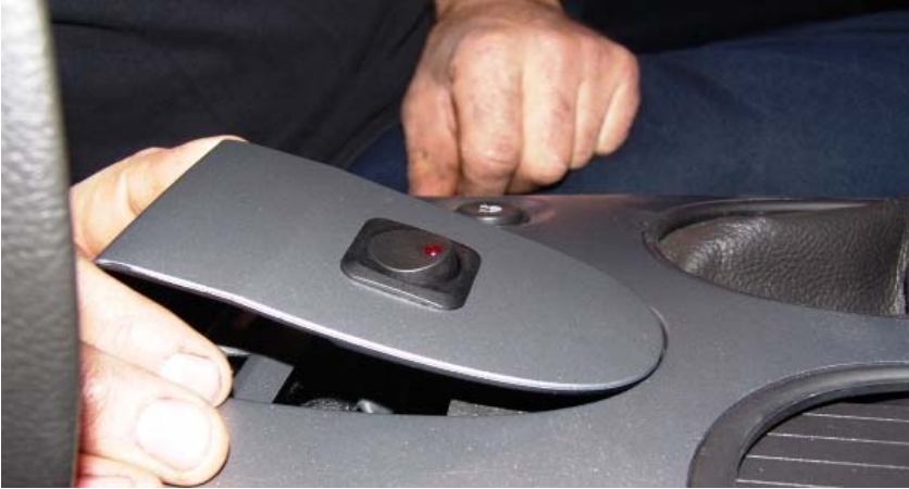
Figure 3: Installing the new trim plate with switch (lighted switch shown)
