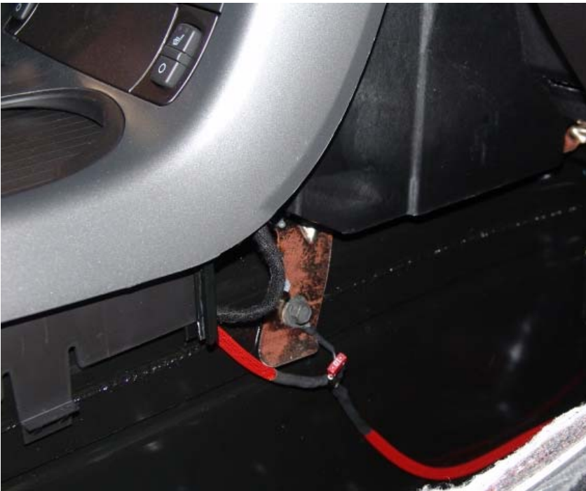
Figure 4: Installing the ground strap
