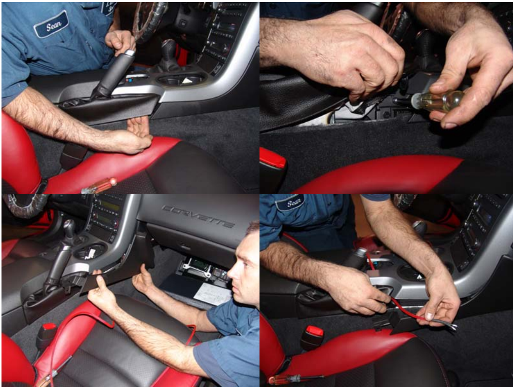
Figure 2: Removal of parking brake boot and side trim panel.
