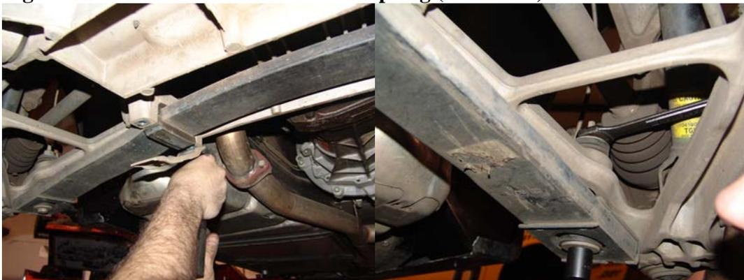
Now that the spring has been removed, take the upper shock mounts loose from the car and remove the rear shocks. This is done by removing the two 10mm bolts holding the upper shock mount plate to the frame of the car.
