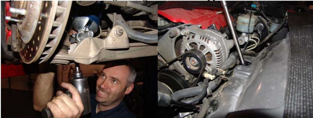
Once both coil overs are installed, tighten the upper shock mount at the frame. The shock will want to turn while doing this, make sure that the bolt holding the shock in place is parallel to the frame once it is tight and not at an angle.
