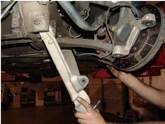
Now that the spring is un-loaded and the shocks have been removed we can focus on the removal of the leaf spring from the car. You will see two plates and four bolts holding this to the car under the center of the K member.
