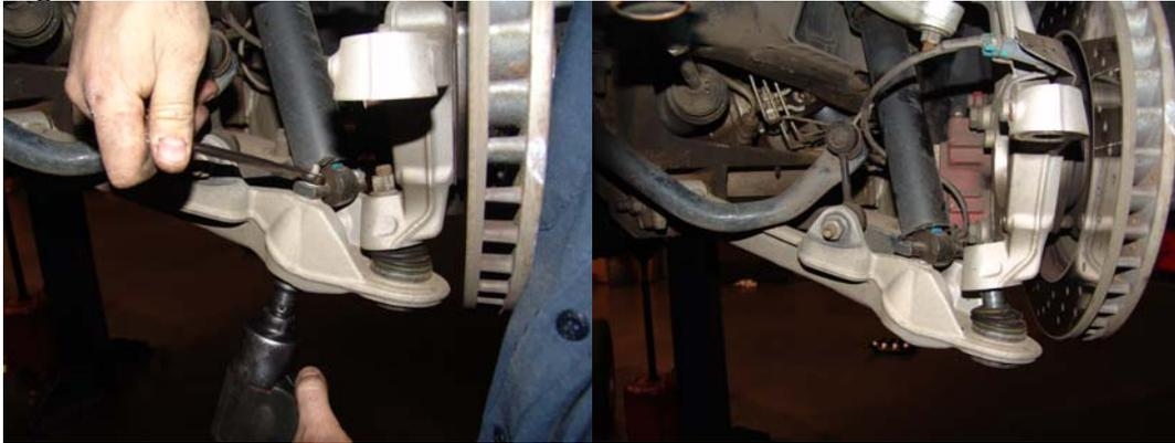
**Figure 5 Separation of the front lower control arm**
