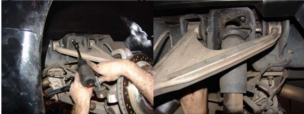
Pull the shock free, and clean off any debris that might be on the frame. We have now completely removed the shock and spring system from the car and are ready to install our new LG coil over suspension package.
