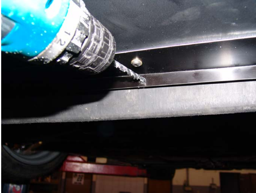
Figure 9: Drilling holes into vertical support
