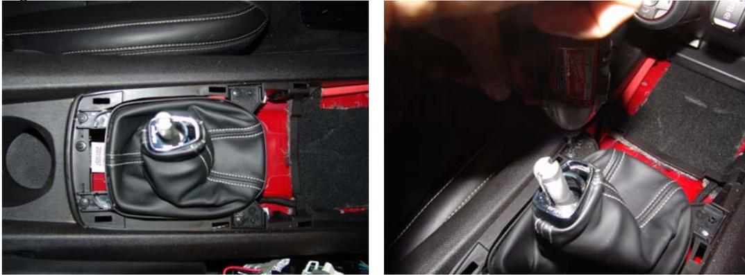
Once the boot has been removed, you will see the shifter and the weather boot under as shown below
