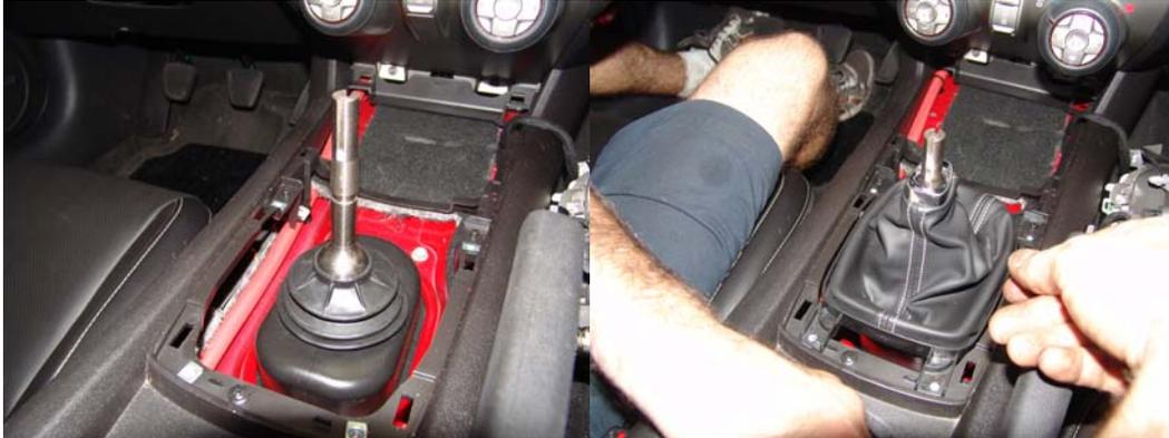
**Figure 13a and 13b: Install of shifter knob**
