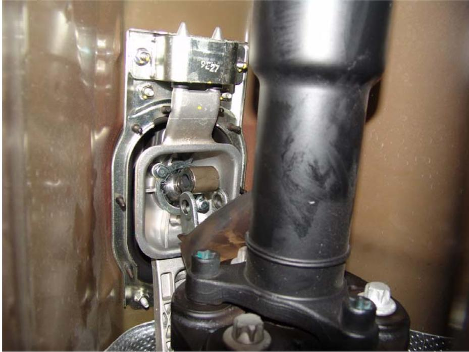
**Figure 8: Shifter bolt removal**
