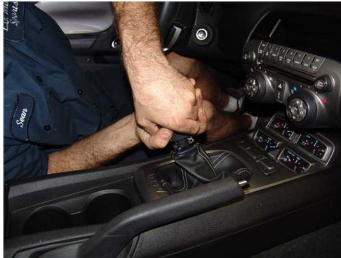
Once the shift knob has been removed you can now remove the lower shifter trim plate from the car. Again this piece is held in with small GM clips. You may find it easier to use a small flat blade screw driver, or clip removal tool. See figures 2a and 2b.
