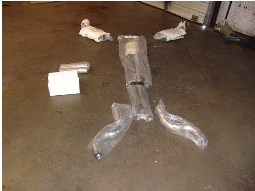
Figure 12: Rear S pipes, X pipe, mid section and optional mufflers
