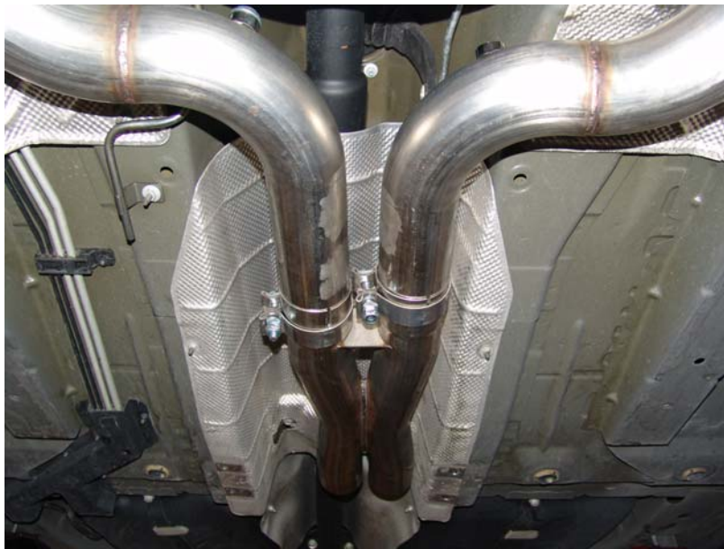
Figure 16: install of X pipe onto S pipes.
