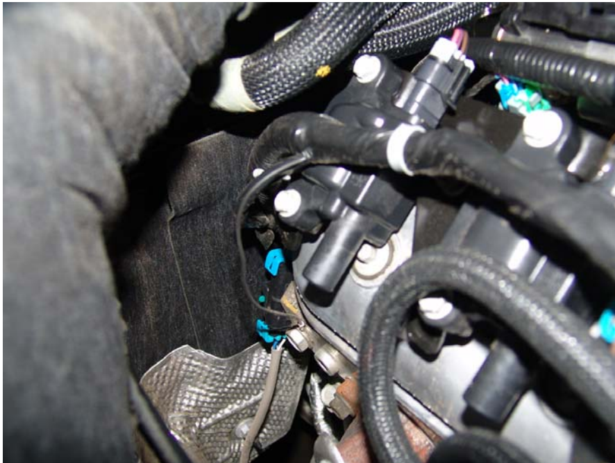
Figure 6: Passenger side front O2 sensor location
