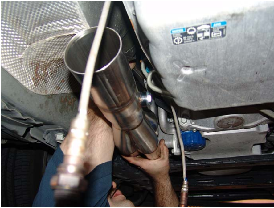
Figure 9: Install of Driver side header
