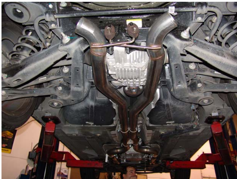
Figure 17: Rear mid section installed into rear hangers.
