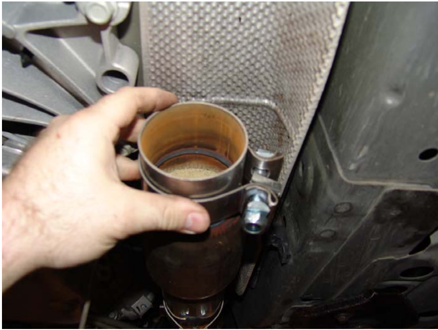
Figure 14: High flow cat installed with 3" clamp
