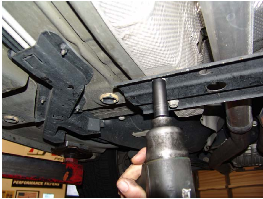
Figure 2: Center tunnel brace removal.
