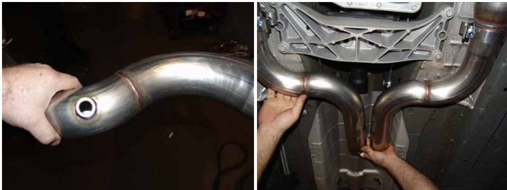
Figure 15: S pipe being installed with rear O2 sensors.
