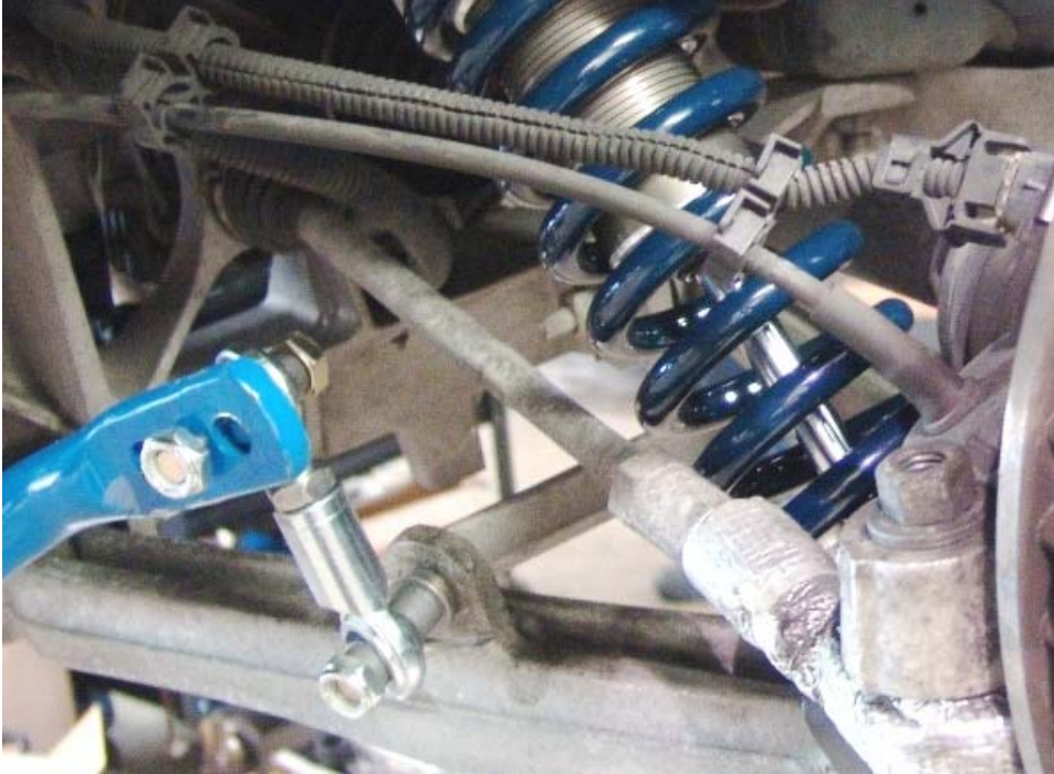
Figure 3: Rear end link installed
