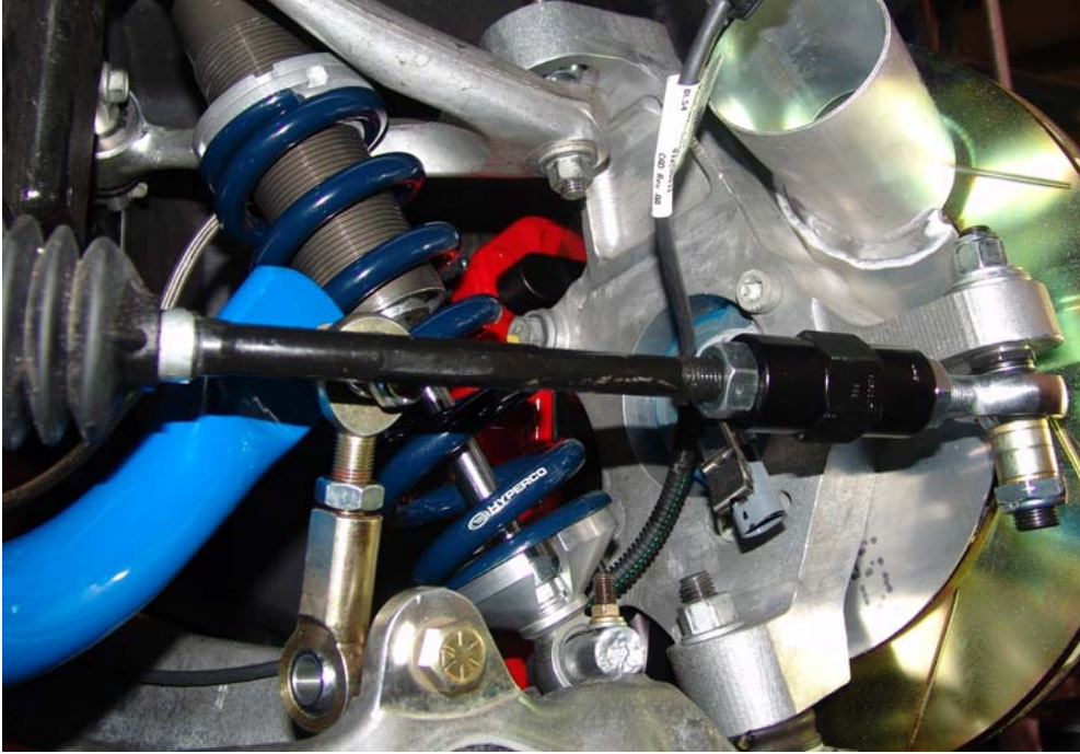
Figure 1: Front end link being installed (shown with optional LG coil overs, G1 sway bars, billet drop spindles, and spindle ducts)
