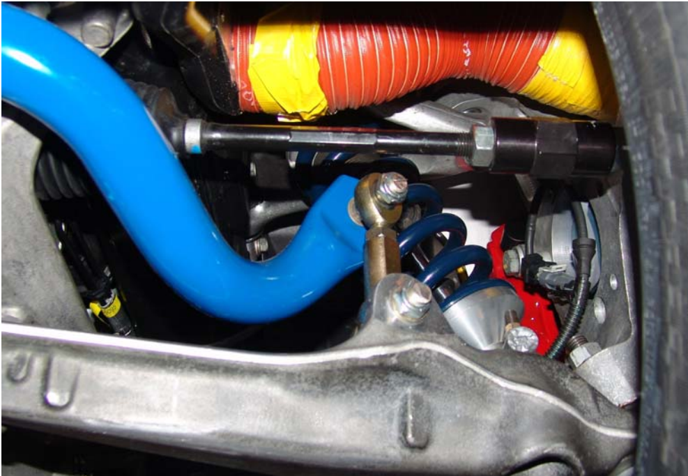
Figure 2: Front link installed
