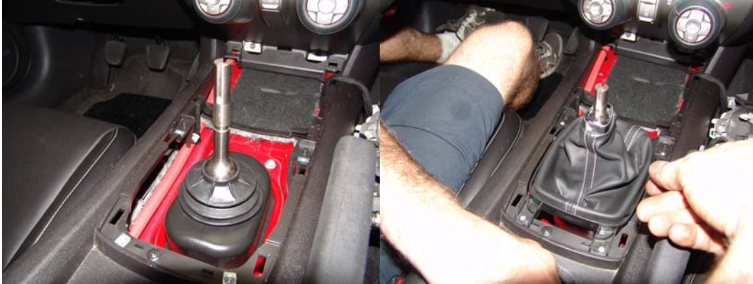
Figure 12a and 12b: New shifter install and boot replacement
