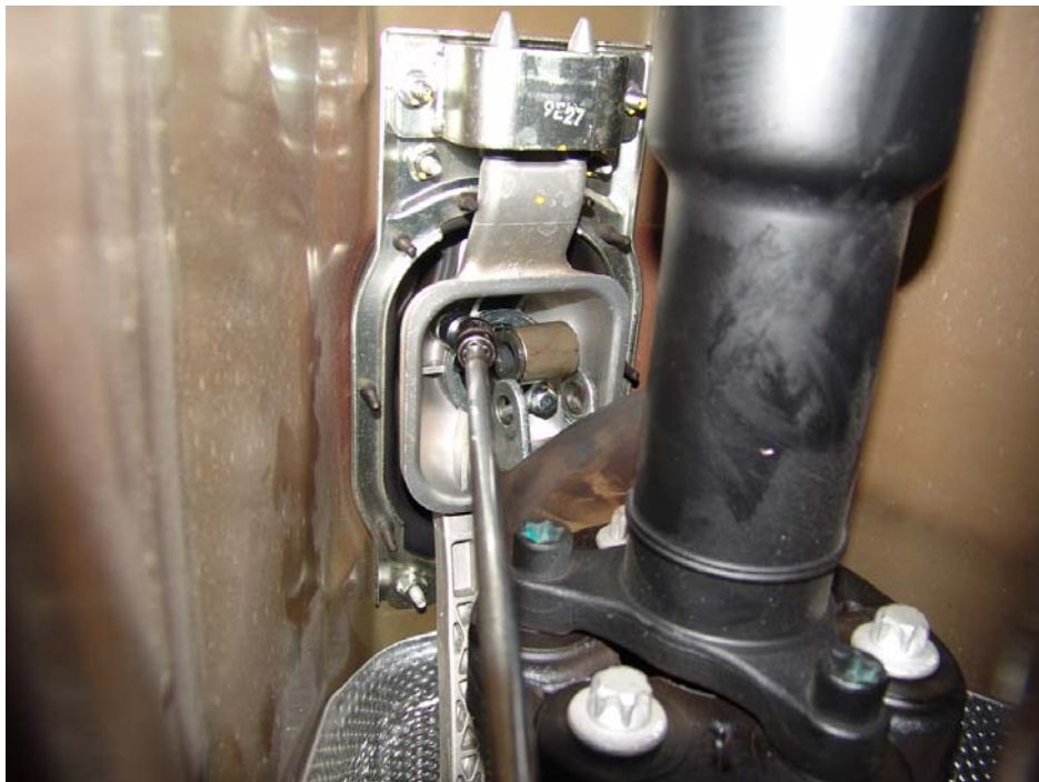
Figure 8: Shifter bolt removal
