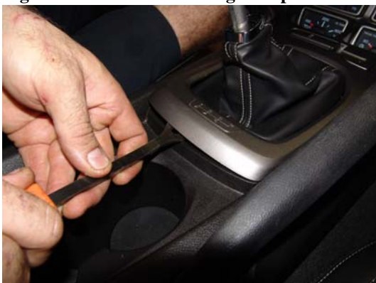
Figures 2a and 2b: removing trim panel
