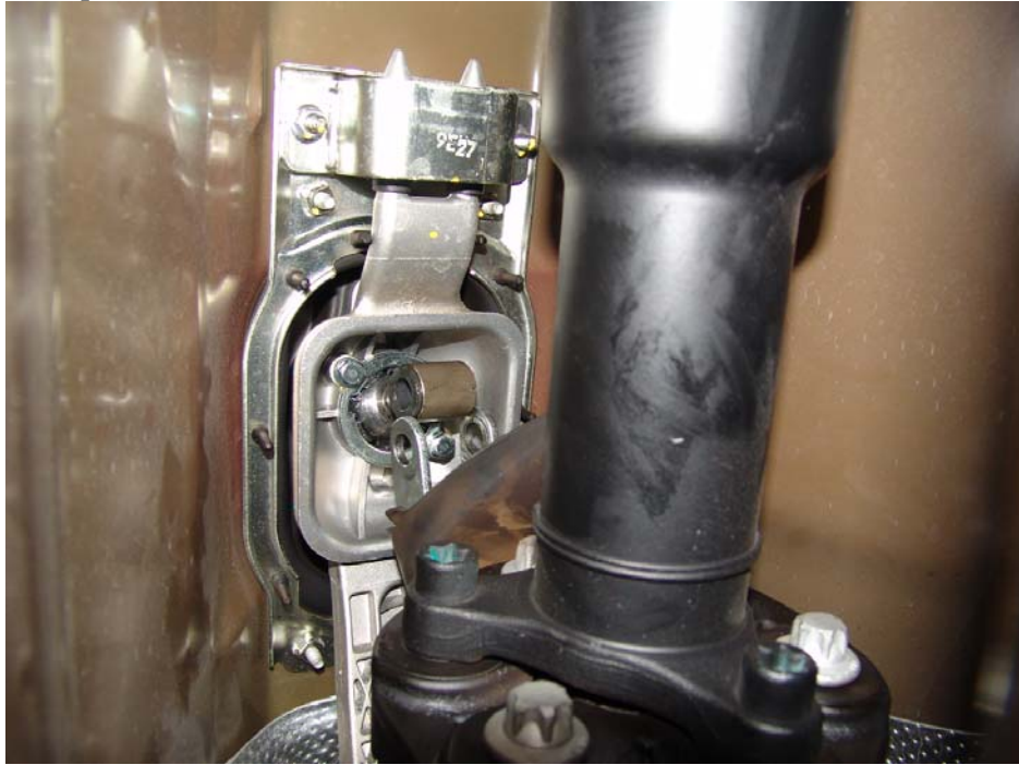
Figure 7: Pivot pin removal
