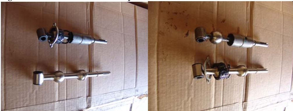
Figure 11: Stock and LG shifter side by side.
