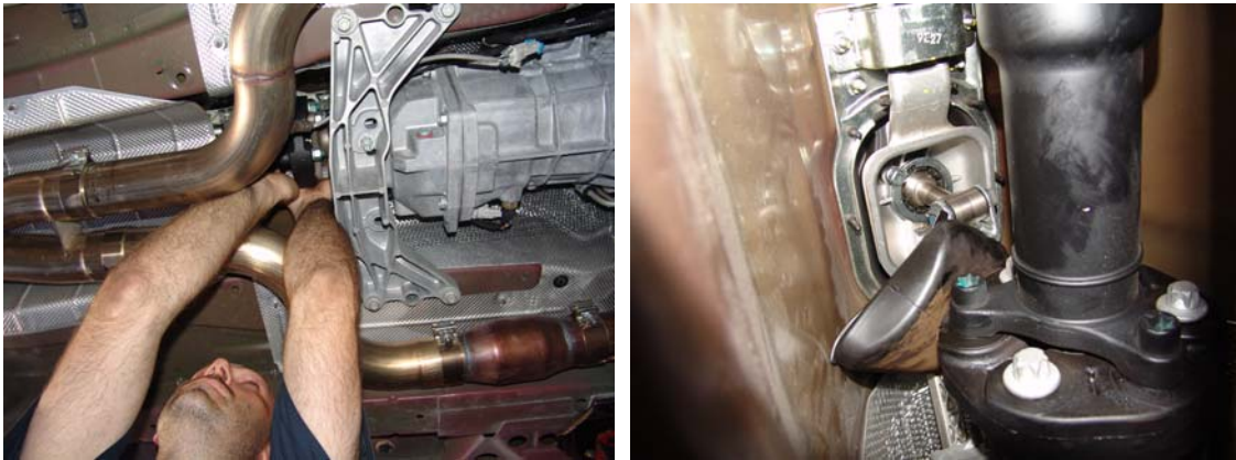
Figure 5a and 5b: removing dust boot and pivot rod
