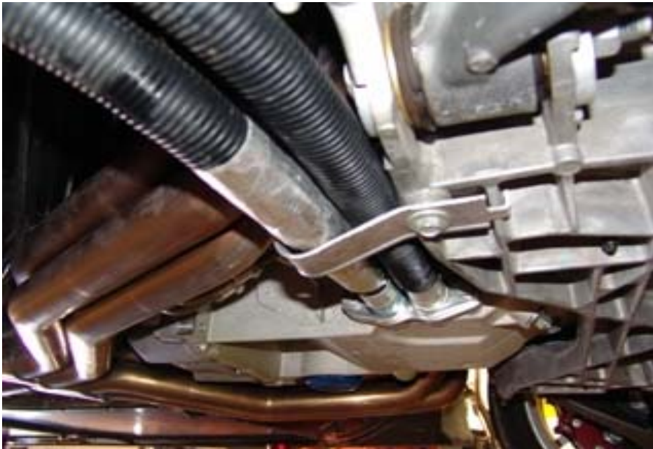
Figure 1: Oil line clearance after bracket has been bent.
