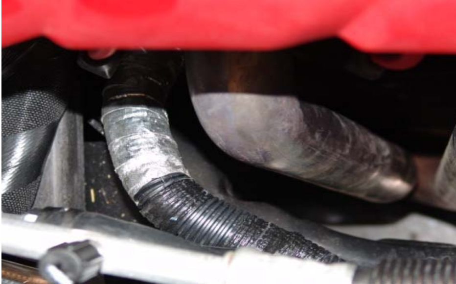
Figure 2: Passenger side wiring harness after being relocated
