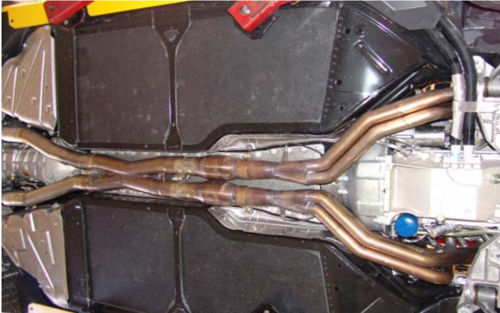
Figure 5: Fully installed LG Long Tube header system on 2006 Z06.
