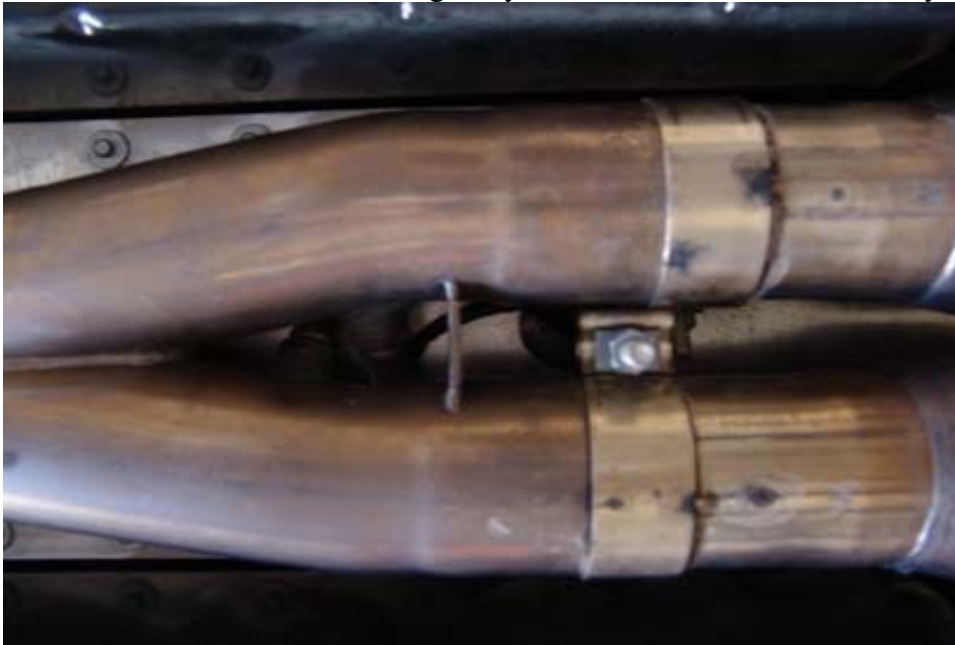
Figure 4: X-pipe location with hole drilled for O2 sensor wires (front is to the right).
