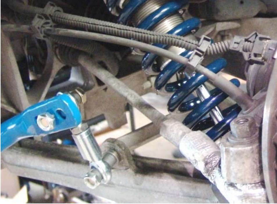
Figure 3: Rear end link installed
