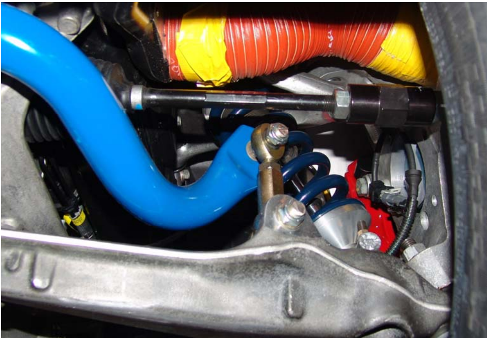
Figure 2: Front link installed
