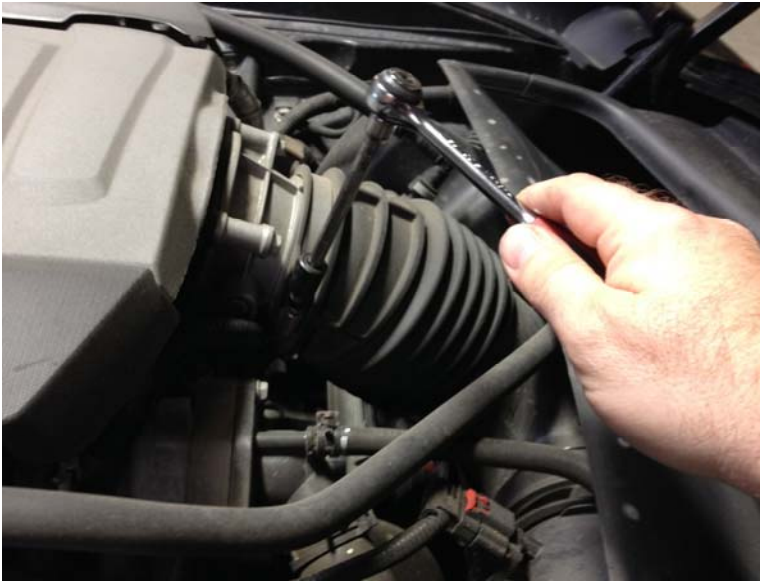
Figure 4: Removing the hose to TB
