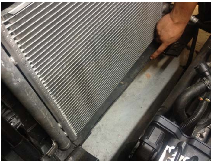
Figure 10: lower splash guard trimmed.
