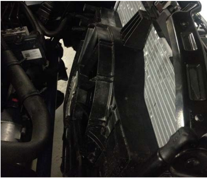
Figure 6: fan and radiator after chimney and inlet box removed.
