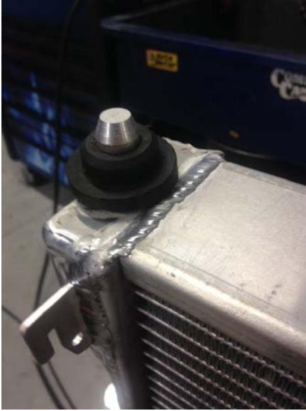
Figure 11: trimmed support cup installed
