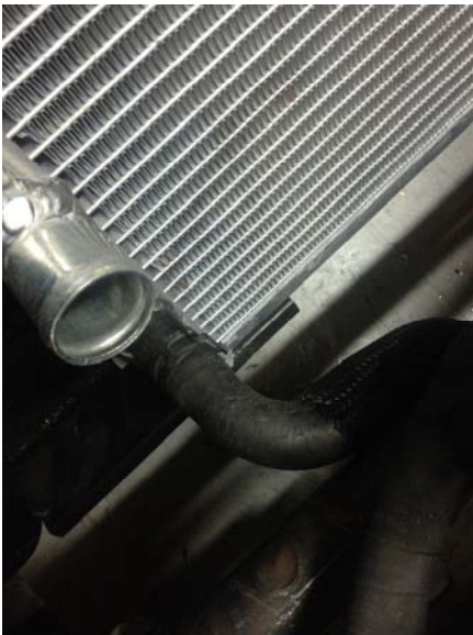
Figure 12: oil cooler water line
