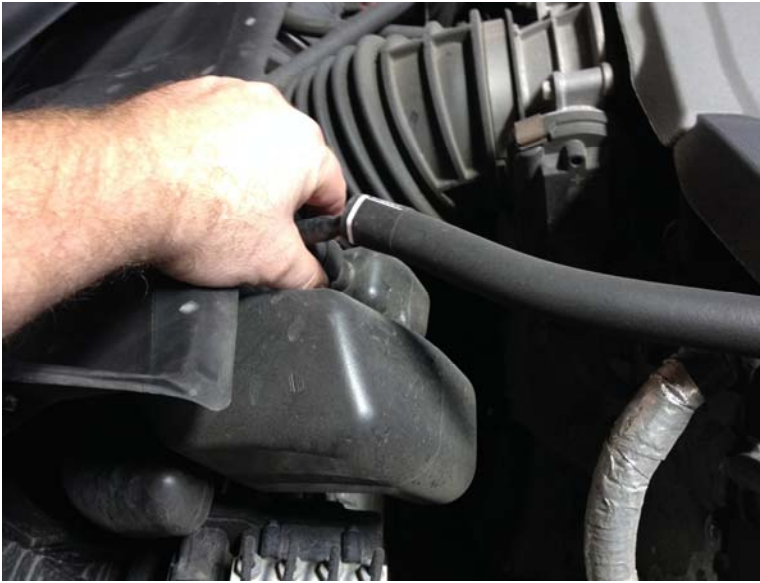
Figure 2: removing PCV lines
