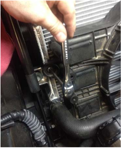
Figure 14: install screws into fan assembly
