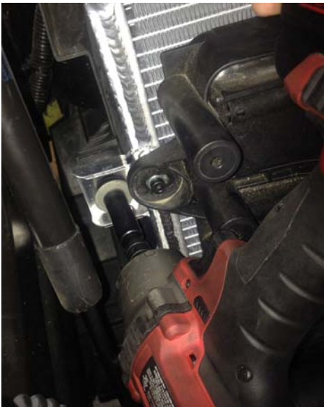
Figure 15: install bolts into radiator sides
