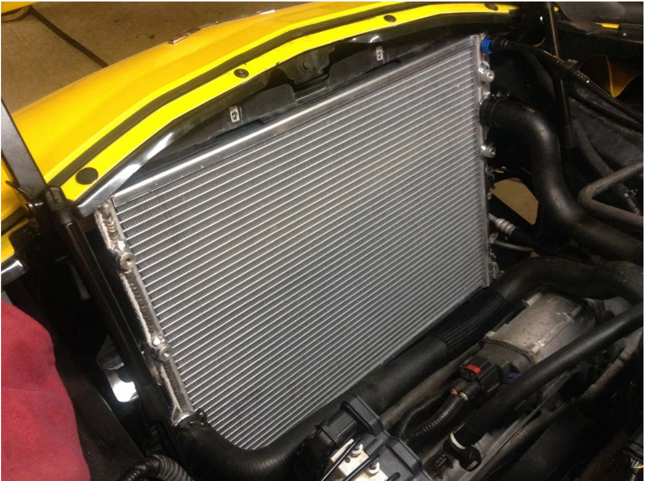
Figure 13: Radiator installed and hoses connected.
