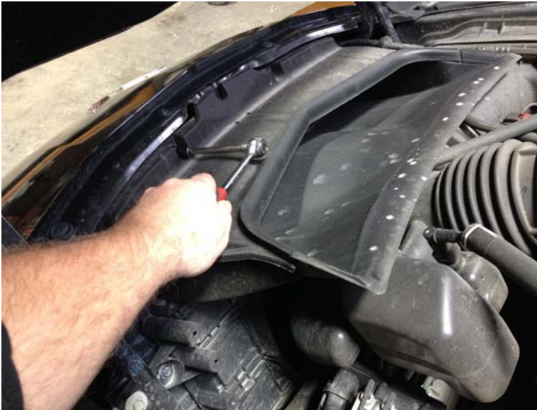
Figure 1: removing chimney from radiator
