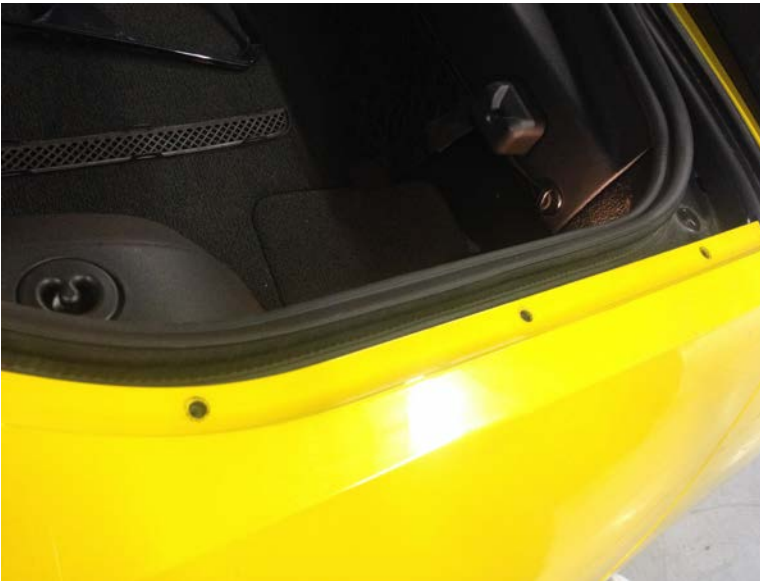
Figure 7: bolts inside trunk lip
