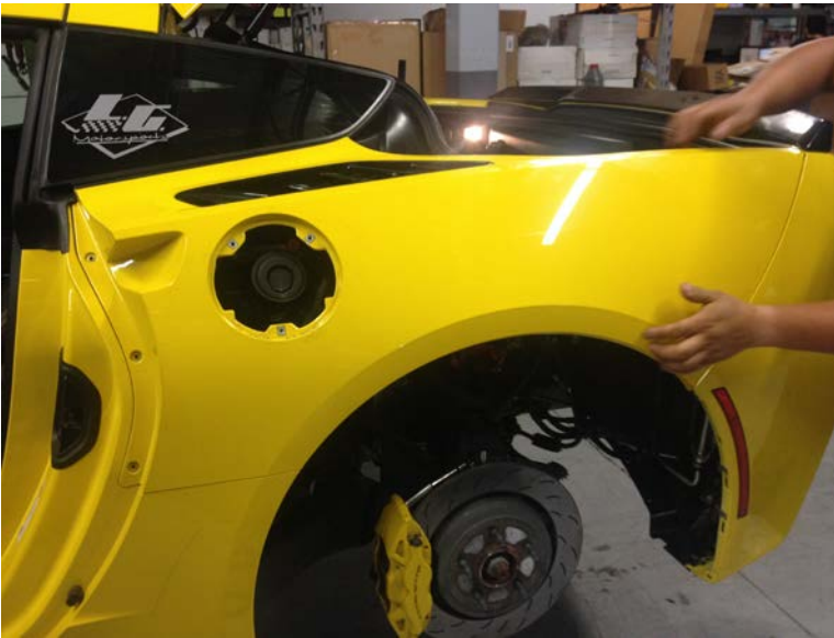
Figure 11: All bolts and inner panels removed
