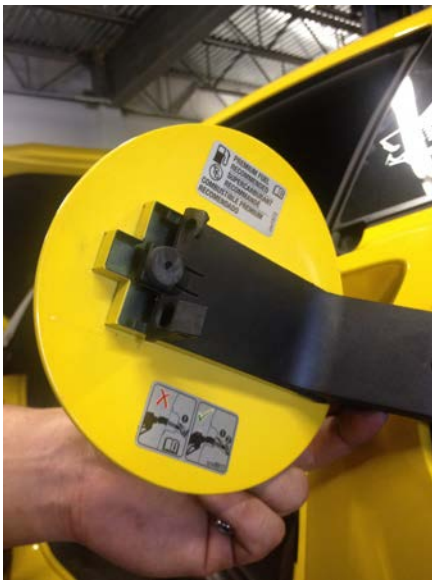
Figure 1: Removing gas door
