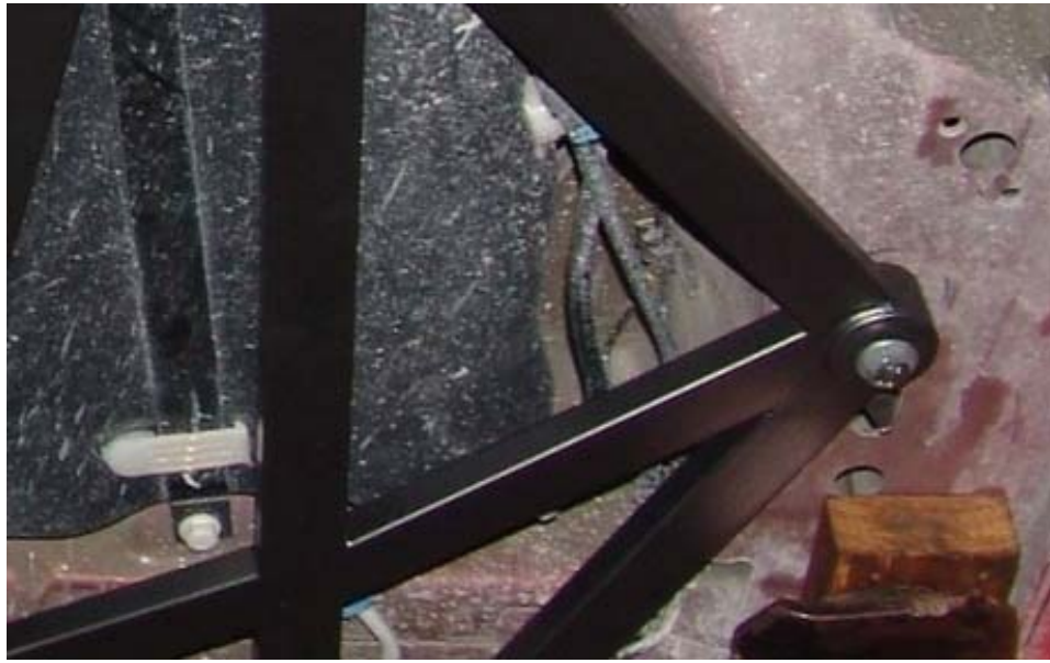
Figure 6: Outer brace bolt installed
