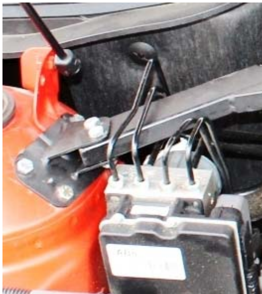
Figure 3: Passenger mount and ABS lines
