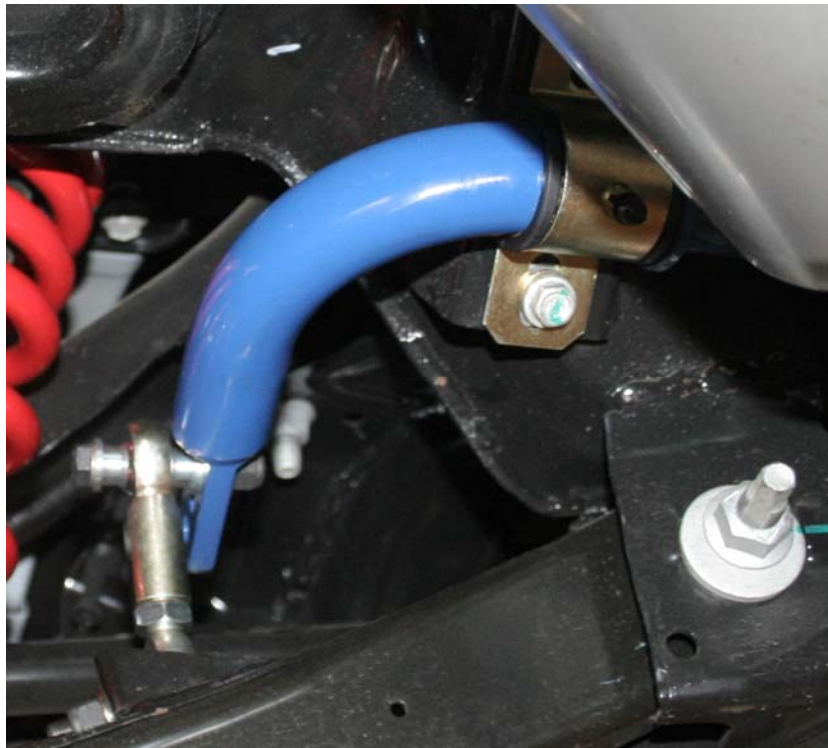
Figure 4: Close up of sway bar installed with bushings and links
