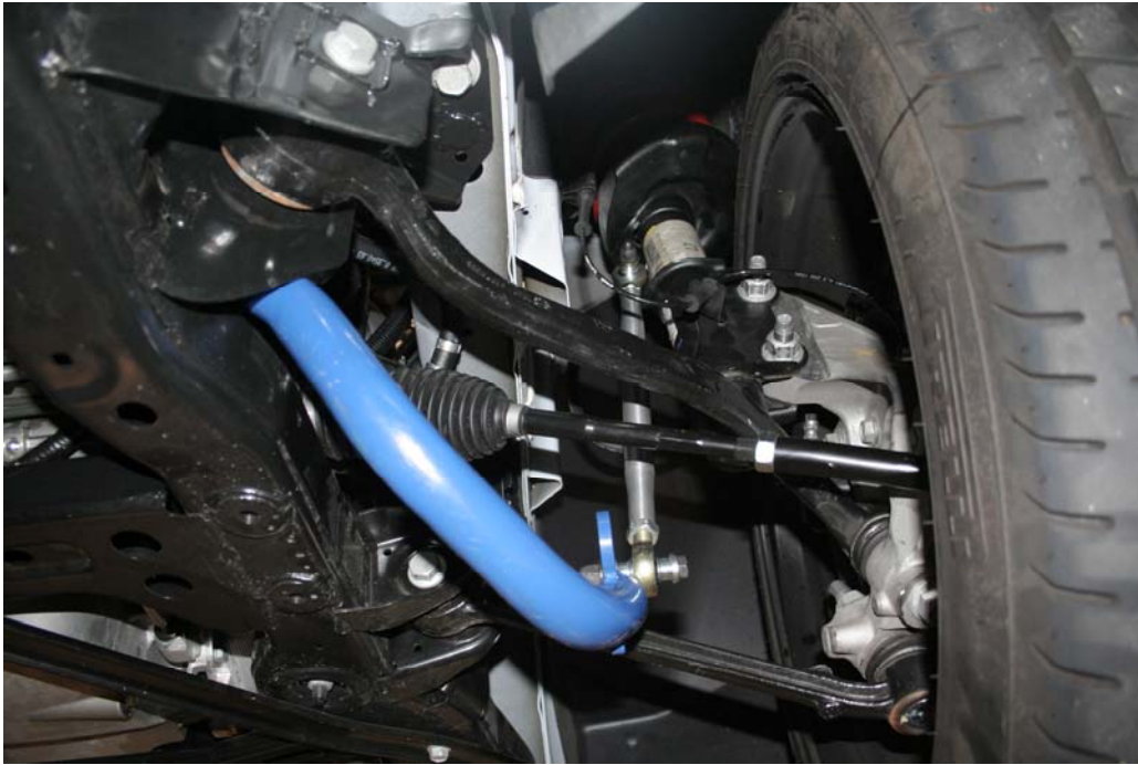
Figure 6: Front sway bar installed (with HD links installed)
