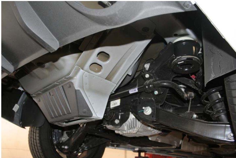
Figure 1: Rear sway bar removal.
