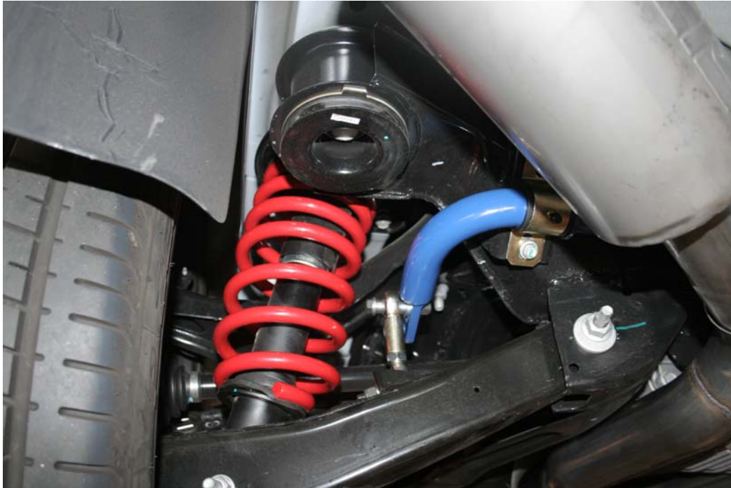
Figure 5: New rear sway bar installed, shown with optional HD links and Super Springs
