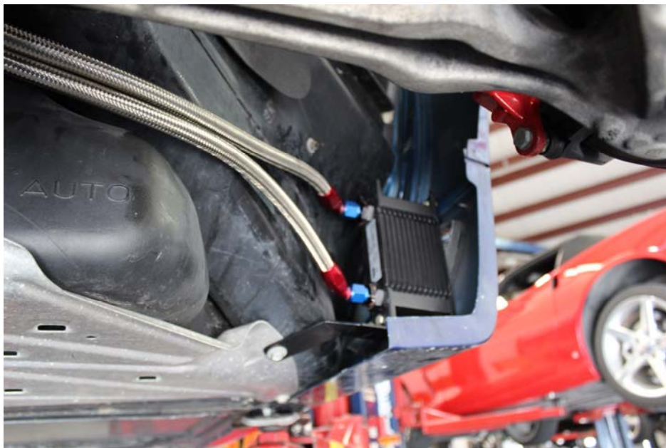
Figure 6: Passenger side cooler mounted
