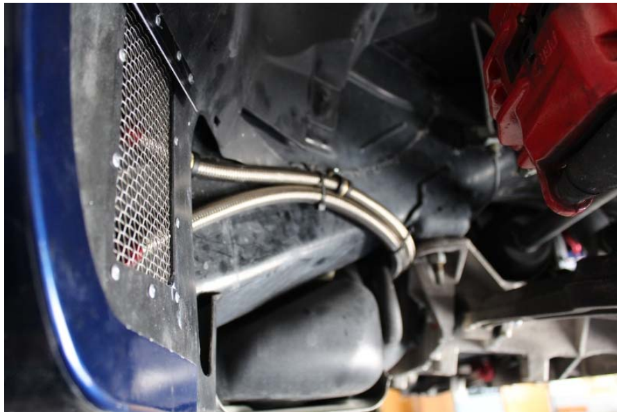
Figure 8: Driver side cooler and screen installed
