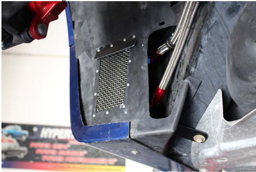
Figure 7: Driver side cooler and screen installed
