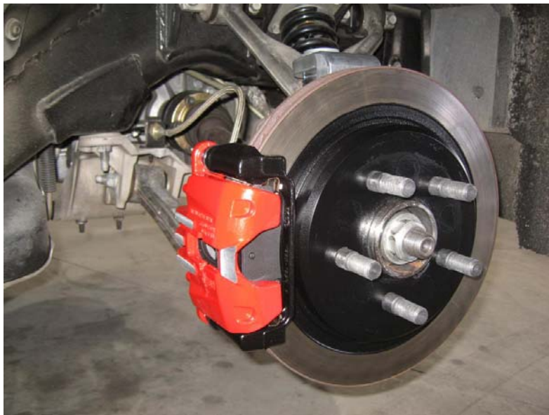
Figure 7: Rear drag spindle installed with brakes
