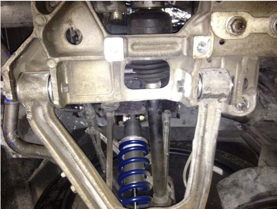
Figure 10: Rear lower arm finished and installed (notice inserts from outside in.)
