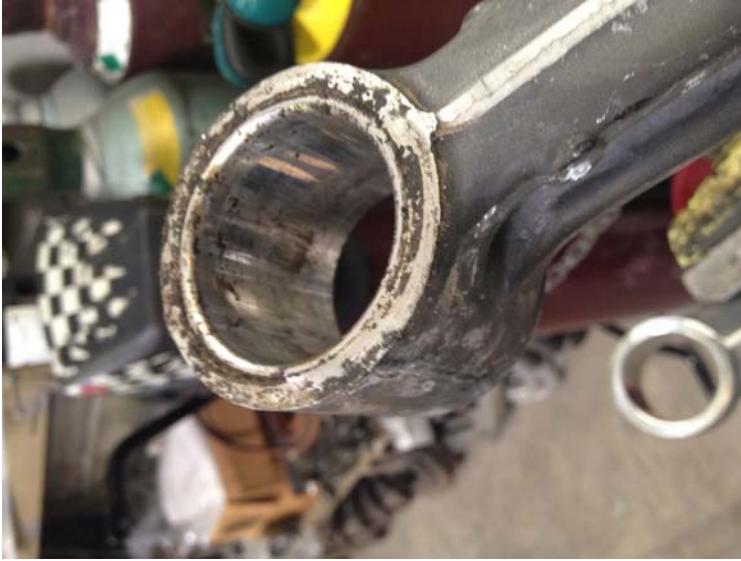
Figure 1: Bushing removed before cleaning
