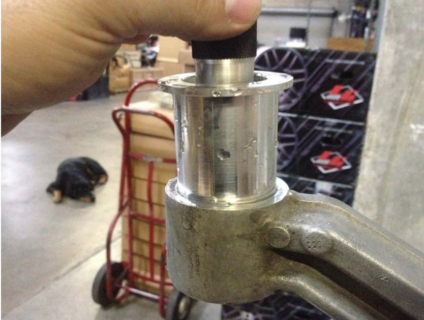
Figure 7: Installing into control arm.
