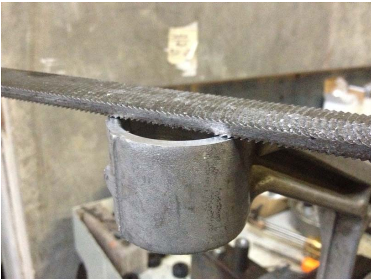
Figure 4: Removing material on flange end.
