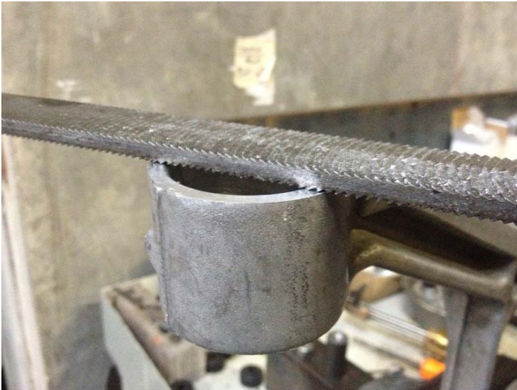
Figure 4: Removing material on flange end.
