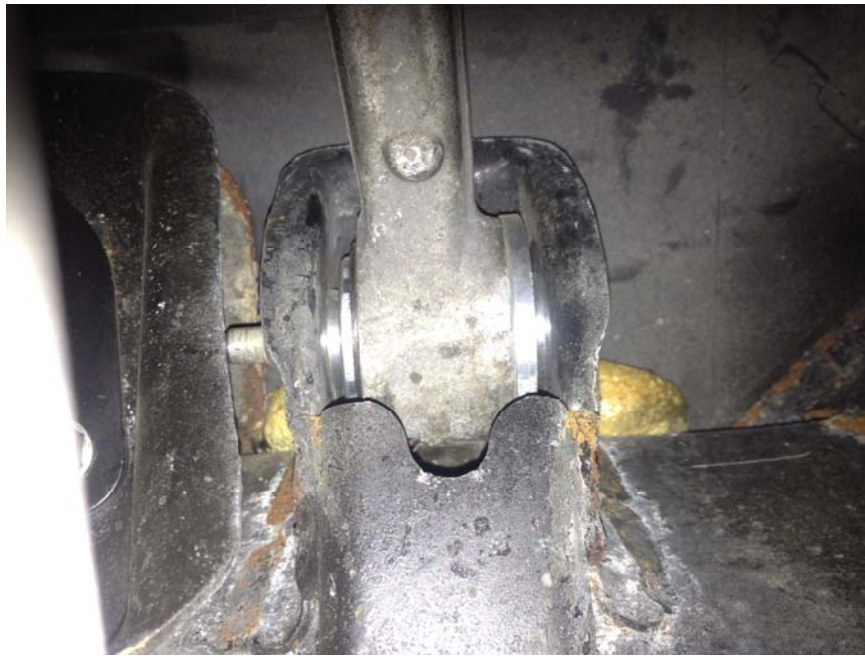
Figure 13: Rear upper arm installed
