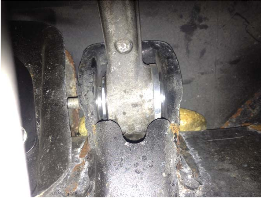
Figure 13: Rear upper arm installed
