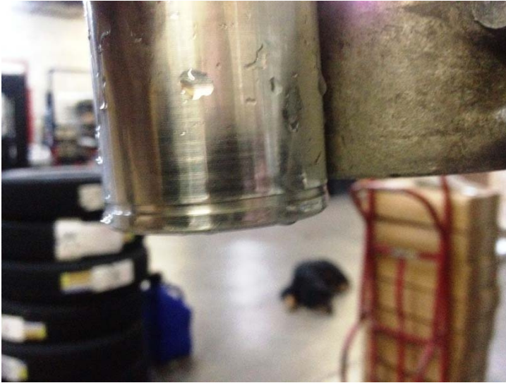
Figure 4: Checking for C-clip clearance
