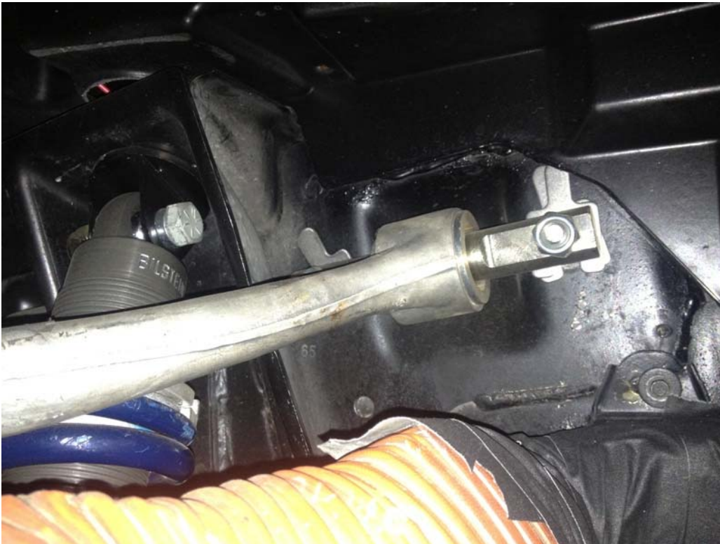
Figure 12: Front upper control arm installed
