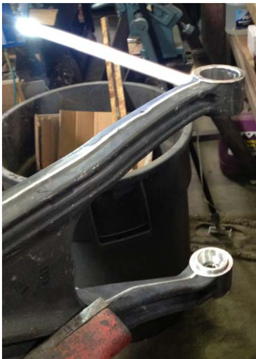
Figure 6: Heating control arm ends
