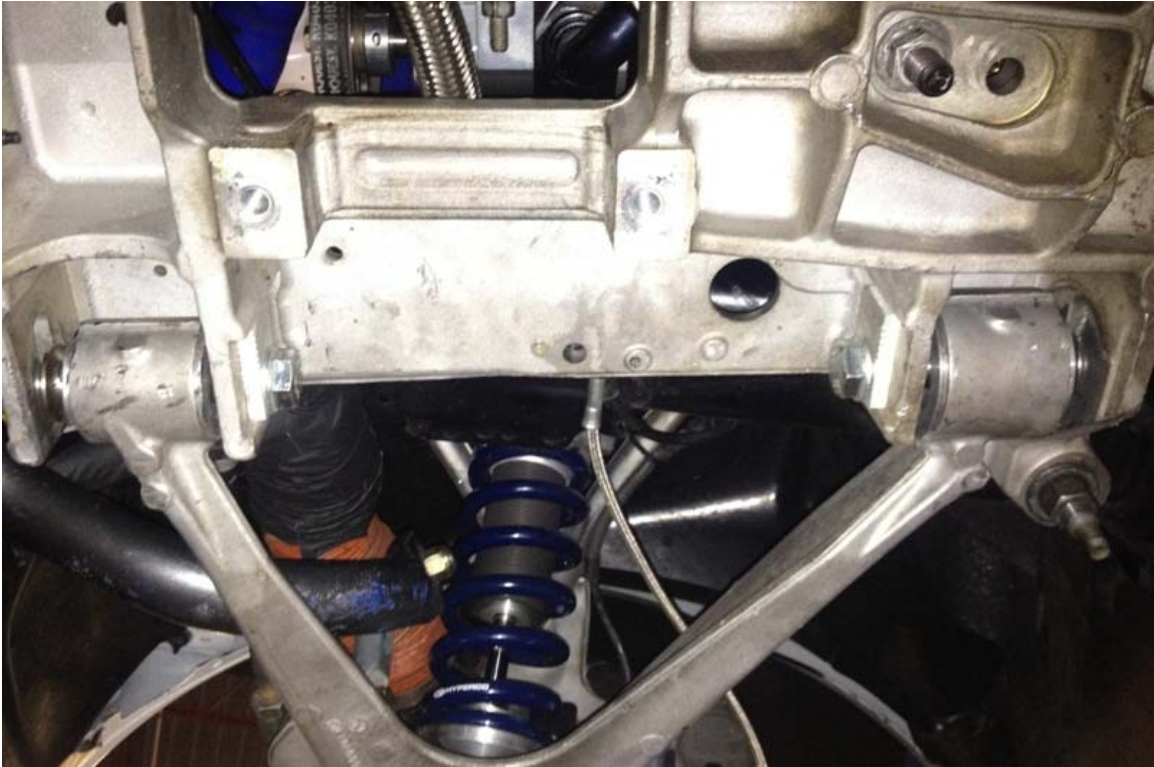
Figure 11: Front lower arm installed (notice housings inserted from the inside out)
