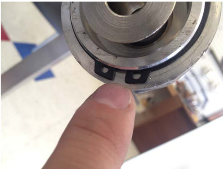
Figure 8: External C clip installed
