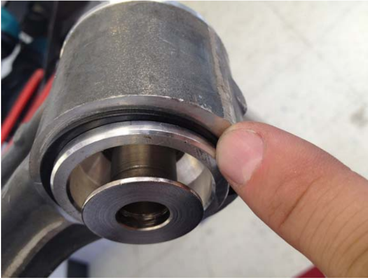
Figure 9: Make sure the clip is seated into the groove
